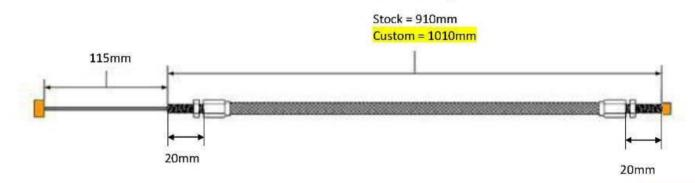
Threaded adjuster with one jam nut
